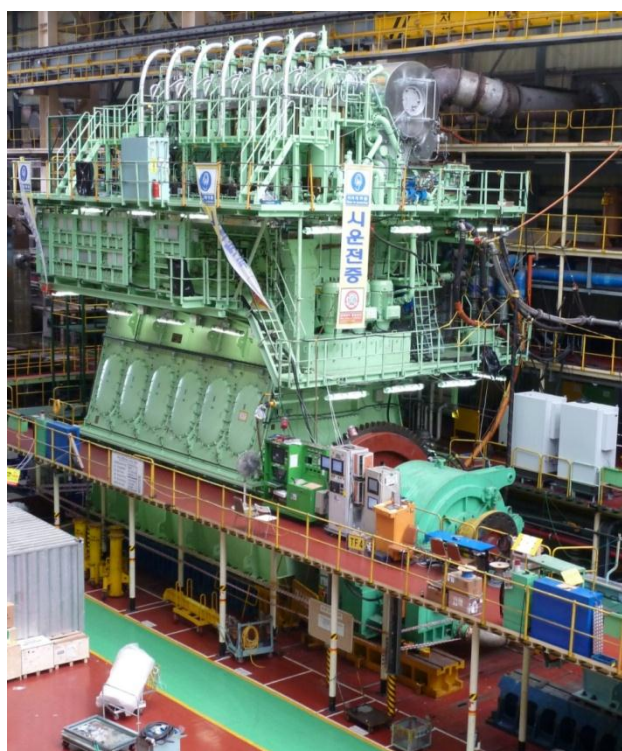
Figure 4: 23 MW low-speed engine with Tier III EGR at Hyundai Heavy Industries test bed 2012
