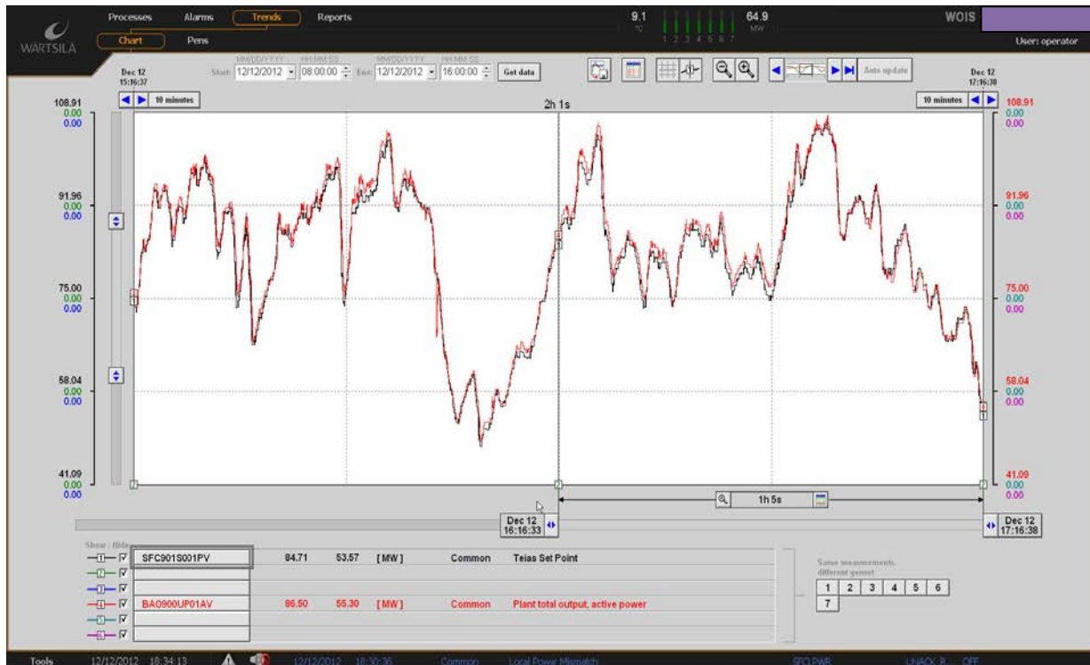
Figure 1: Gas Engine Power Plant consisting of 7 engine units, 130 MWe, 2 hour Power Plant SCADA Trend. Plant set point signal from the Grid, TSO is typically 40-110 MW in this case.
