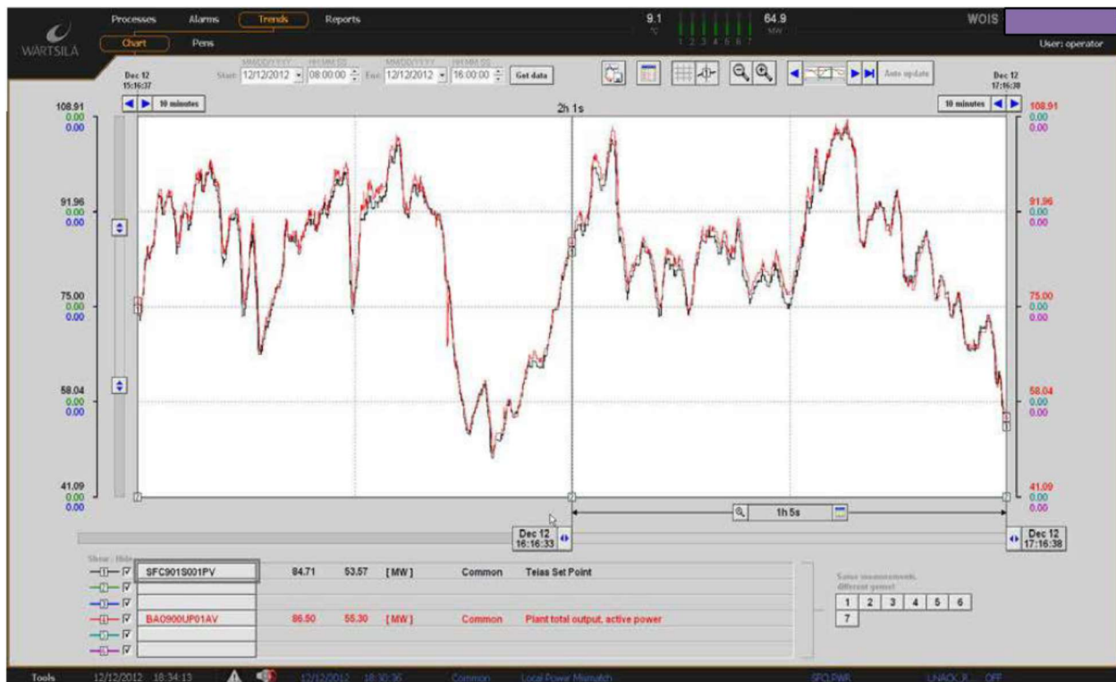
Figure 1: Gas Engine Plant consisting of 7 engine units, 130 MWe, 2 hour Scada trend. Plant set point signal from the grid TSO, is typically 40 -100 MWe in this case. /11/.
